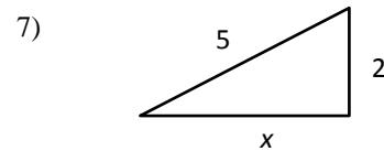
$$\begin{aligned} x^2 + 2^2 &= 5^2 \\ x^2 + 4 &= 25 \\ x^2 &= 25 - 4 \\ x^2 &= 21 \\ x &= \sqrt{21} \\ x &= 4.6 \end{aligned}$$
