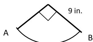
$$\begin{aligned} C &= 3.14 \bullet 18 = 56.52 \text{ in} \\ 56.52 \div 4 &= 14.13 \text{ in} \end{aligned}$$
