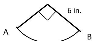
$$\begin{aligned} C &= 3.14 \bullet 12 = 37.68 \text{ in} \\ 37.68 &\div 4 = 9.42 \text{ in} \end{aligned}$$
